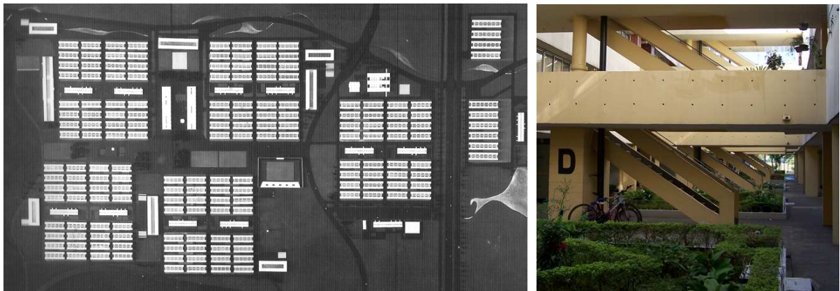
Figure 7 and 8 Zezinho Magalhães Prado Housing Complex · João Vilanova Artigas + Paulo Mendes da Rocha + Fabio Penteadó · 1967. Original sketch of site plan and actual view. Project area: 130 ha; Number of housing units: 10.560 (built 4.680 units); Projected population: approximately 55.000 inhabitants; Density: 81 unit / ha; Developer: Caixa Estatal de Casas para o Povo (CECAP).
